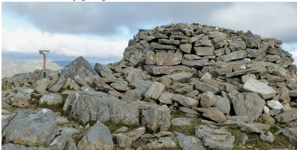
Surveying the summit of Chno Dearg. The top of the rock to the right of the pole was the point measured, but a higher embedded rock could be buried beneath the cairn.
